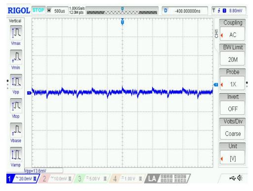
Vout = 1.2V Transient 0.15A to 0.2A@2.5 A/us Vpp = 13.6 mV L = 10 uH and C = 47 uF. f = 571 kHz
