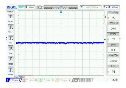
No Load  $V_{PP} = 5.60 \text{ mV}$
