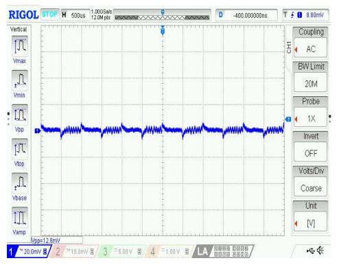
Vout = 1V Transient 0.19A to 0.25A@2.5 A/us Vpp = 12.8 mV L = 10 uH and C = 47 uF. f = 571 kHz
