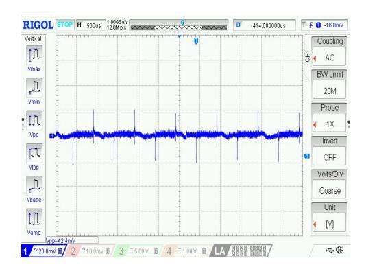
Vout = 1.2V Transient 6.75A – 9A @ 10 A/ $\mu$ s V<sub>PP</sub> = 42.4 mV Fsw = 1 MHz Lout = 0.25  $\mu$ H, Cout = 10 x 47  $\mu$ F
