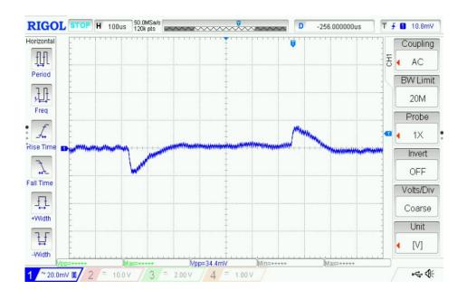
Vout = 1.8V Transient 0.12A to 0.4A@2.5 A/us Vpp = 34.4 mV L = 10 uH and C = 47 uF. f = 571 kHz
