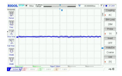
No Load  $V_{PP} = 6.4 \text{ mV}$
