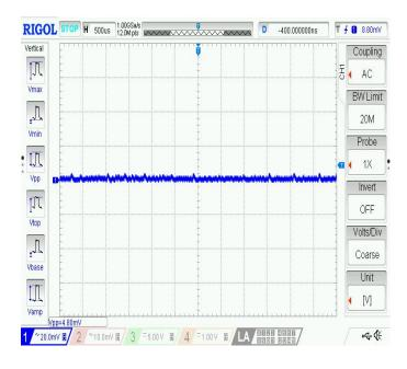
No Load  $V_{PP} = 4.80 \text{ mV}$
