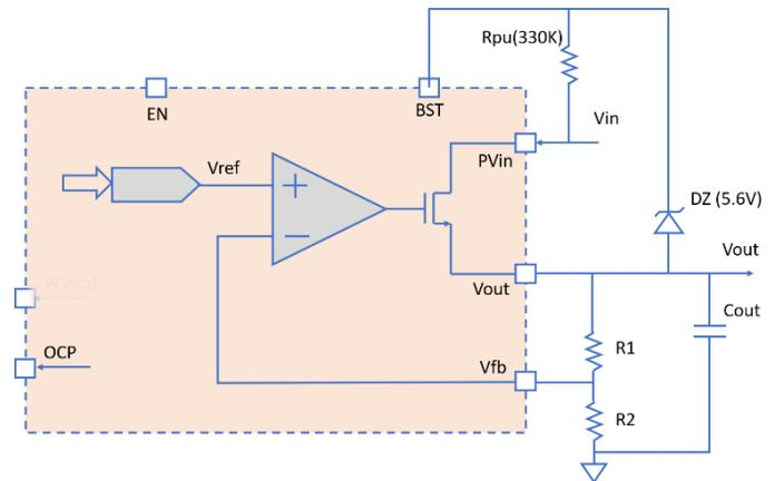
Figure 11: LDO bloc diagram
