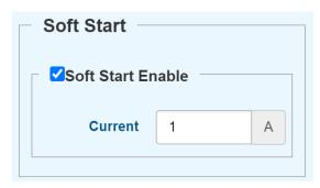
However the C751\_B uses a CV based soft-start and allows the user to program a specific soft-start time independent of Cout. The soft-start time is programmable in the range 0.5ms to 8.0ms.
