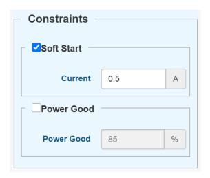
The C750\_B CC based soft start feature allows a controlled ramp of the output based on the value set by  $C_{\text{OUT}}$
