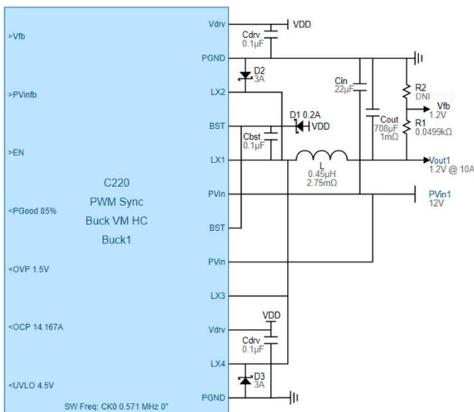
The customizable output voltage is specified by the power engineer during customization using AnDAPT's cloud-based WebAmP development software. The C220 component has customizable control and status pins including enable input, an optional power-good output, and optional output flags to signal when the system triggers an overvoltage (OVP), overcurrent (OCP), or input undervoltage lockout (ViUVLO) condition. The threshold values are specified by the power engineer using the WebAmP tool.
